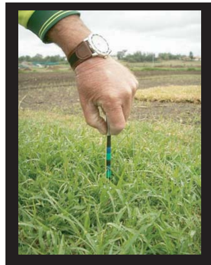
Henry Locock designed this measuring device to allow him to quickly measure if a plot required mowing or not.
